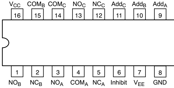
Figure 1. Pin Connection (Top View)
